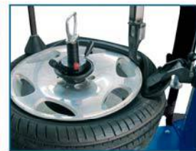
Safe and easy mounting with plastic tool, roller and rotating helper PLUS93
