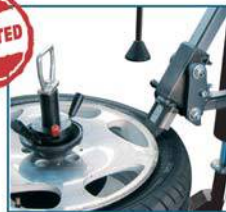
The tool enters between bead and rim
