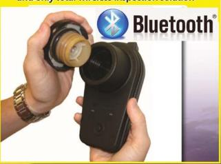
Integrated OBDII DAD Verification and Charging Station to ensure your OBDII DAD is operating, communicating and charging properly
