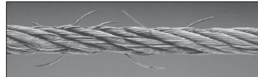
Cable with Broken Wires
