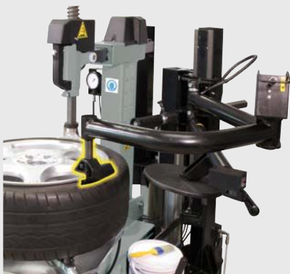
PLUS83D PLUS83 con G800A64 pressore sagomato WDK PLUS83 with G800A64 WDK bead pressure device PLUS83 mit WDK- Wulstniederhalter G800A64 PLUS83 avec outil de pression WDK G800A64 PLUS83 con prensa talón WDK G800A64
