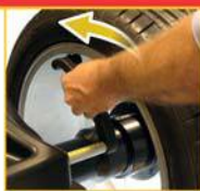
Rim run-out measurement with internal data gauge.
