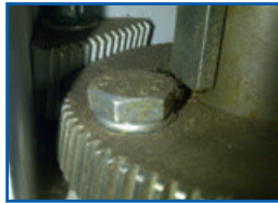
Self-locking conical design
